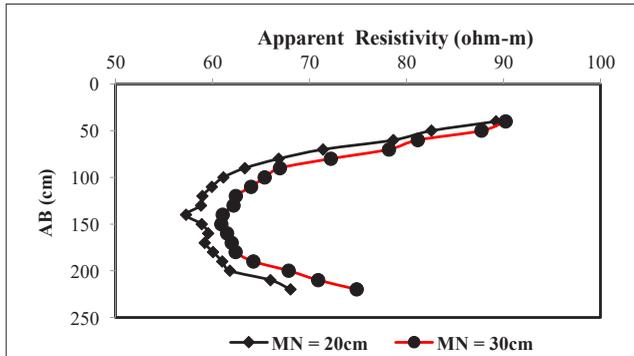
Figure 2: Effect of MN separation on apparent resistivity
