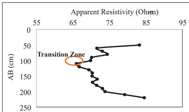
Figure 4: Typical anomaly showing the transition zone in a Schlumberger array
