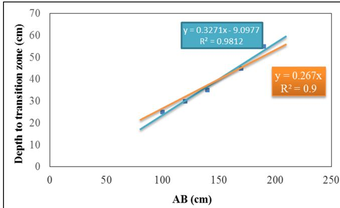
Figure 5: Depth of investigation versus current electrode spacing (AB) using the Schlumberger array
