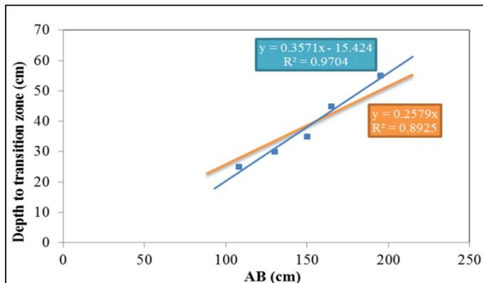
Figure 6: Depth of investigation versus current electrode spacing (AB) using the Wenner array
