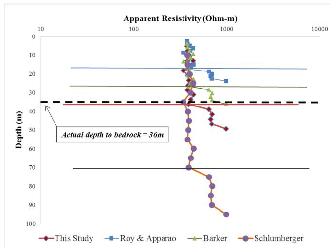
Figure 7: A comparison of estimated depth to bedrock (VES curves) using different depth factors and actual depth to the bedrock from the borehole logs
