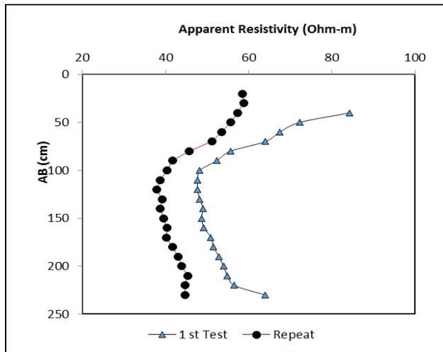
Figure 3: Apparent Resistivity curves (Schlumberger) for depth of 25 cm
